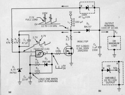
Figure 1 The output voltage of a simple variable-frequency dc/dc step-up converter depends on the device under test's breakdown voltage (a). To use the circuit as a variable
